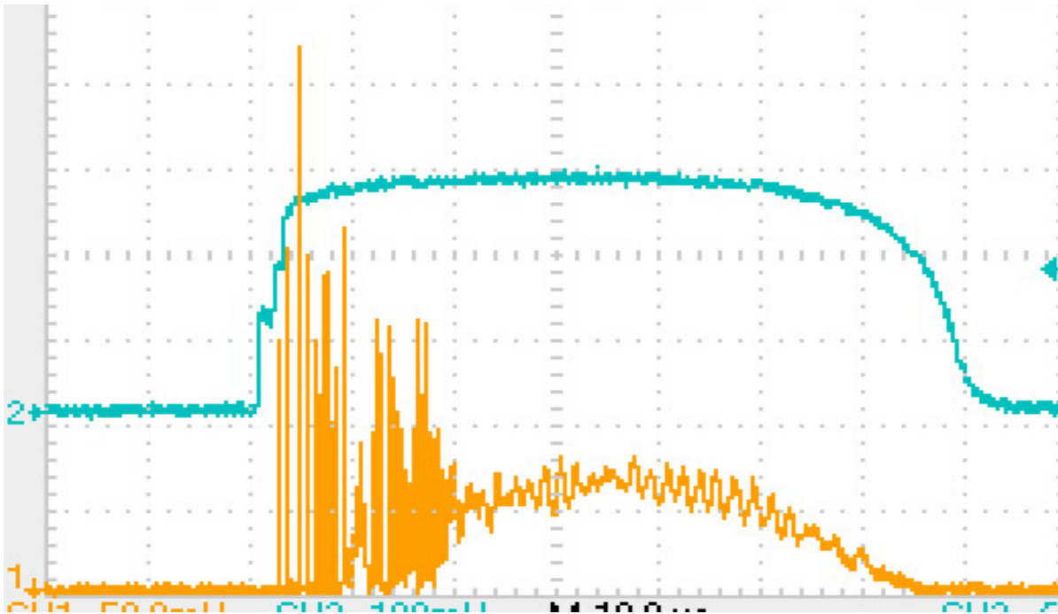
Figure 3-21: Temporal Profile of Cr 3+ :LiSAF Laser Pulse (Cyan) and Ho 3+ :BYF Laser Pulse (Orange) at Maximum Output Energy.
